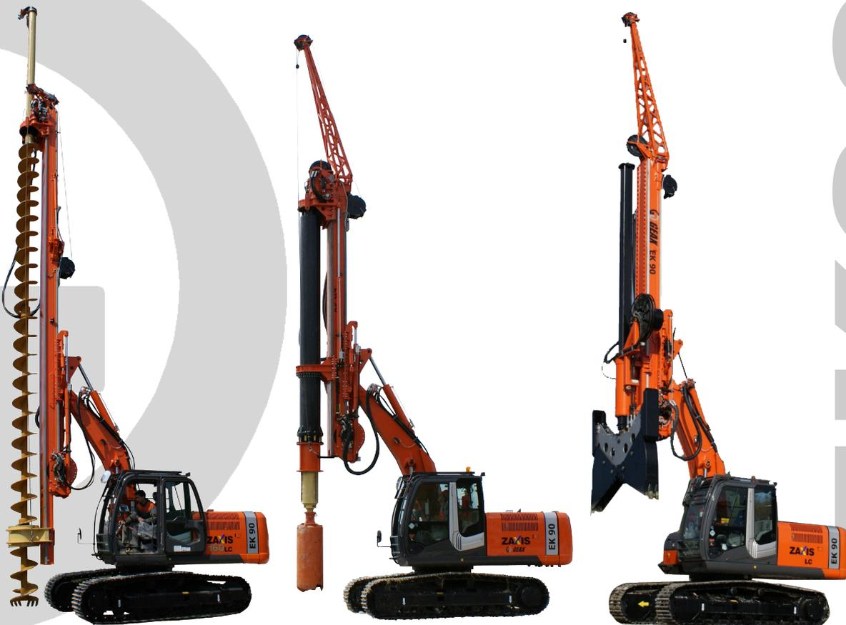
GEAX EK90 (as all the other GEAX machines) is characterized by an articulation architecture similar to a normal excavator, with a long boom in which is attached the mast. This permits a wide range of mast positioning and independent movements for the vertical alignment. Rope paths do not depend on the position of the mast since winches are fixed on it. This architecture, compared with that (usually parallelogram) of other machines, ensures:
